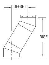
Use to determine the lengths required for an installation. Determine the offset required in view of the obstacles that must be avoided. Refer to the offset/rise chart to determine the elbows required as well as the insulated lengths needed. Check the corresponding offset height dimensions.
