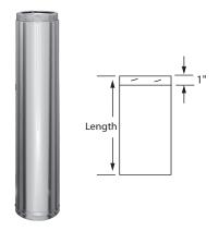
Available in sizes from 5 - to 10-inch diameters, the DuraTech Canada line offers double-wall, 1-inch insulated chimneys. Lengths twist-lock together with just an 1/8th rotation.
