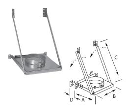
Use to support insulated tee on though-wall chimney installation For installation versatility and convenience, tee can be placed above or below the support. Can also be used as a wall support or re-support. Adjustable arms and sliding base plate are factory-set to ensure minimum clearance of 2". Allows for 2" - 7" clearance to combustibles.
