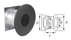
Designed to protect surrounding combustible materials when a chimney passes through a wall. Thimble works with wall thicknesses from 7" up to 12-1/2". Can be trimmed for use with thinner walls. Includes painted Decorative Collar for interior finish. Insulated to prevent heat loss or cold air intrusion.
