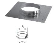
Use to support the chimney on a slab, floor, or joist. It includes a tightening collar that locks around the chimney and is secured by self-tapping screws (included). The collar rests on a horizontal plate screwed or nailed to the floor or slab. It can also serve as an intermediate support. Refer to chart for load bearing capacity.
