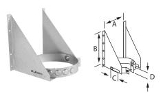
Use to support the chimney on a vertical wall. The triangular plates allow for a 2 ¾" adjustment of the support to the vertical surface. This support can also be used as a wall support above the insulated tee or as a support for an offset elbow. Refer to chart for load bearing capacity. In shorter chimney stack applications, the Wall-Support can also be used in place of a Tee Support. Universal design works with 5", 6", 7", or 8" pipe diameters.
